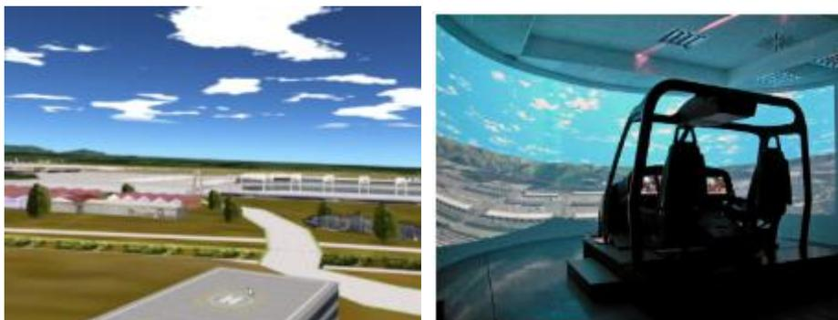
**Out of the window and landing site (top) and view of the engineering simulator (bottom) used for demonstrating T/R low noise IFR procedures in TP2B.**
