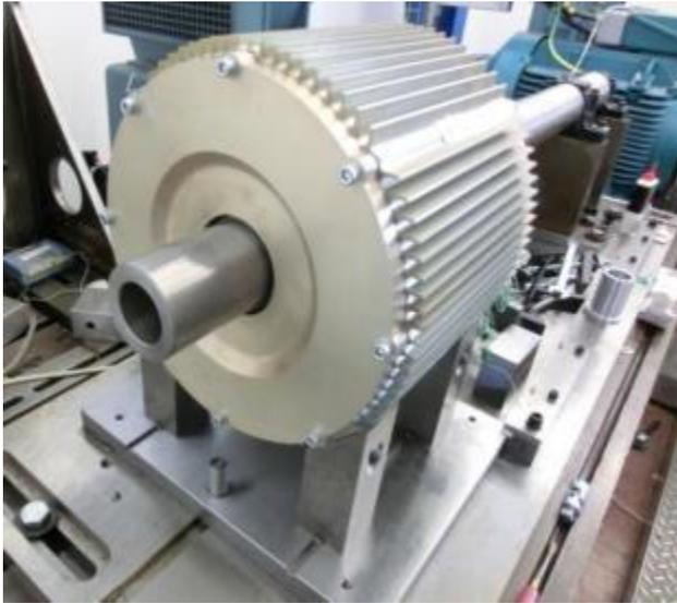
*Electric Tail Drive ELETAD Prototype Radial Motor*
