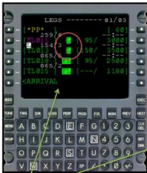
LNA module integrated in the FMS has computed Low Noise trajectories profiles (green labels)
