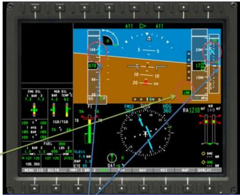
Real Time guidance: Bugs to follow are provided to the pilot in the Speed and ROD indicators
