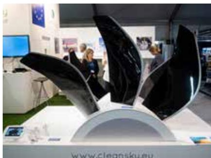
Full-scale Open Rotor Propeller Section
