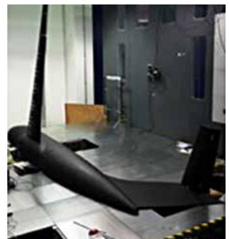
**Model installed in the WT test section**
