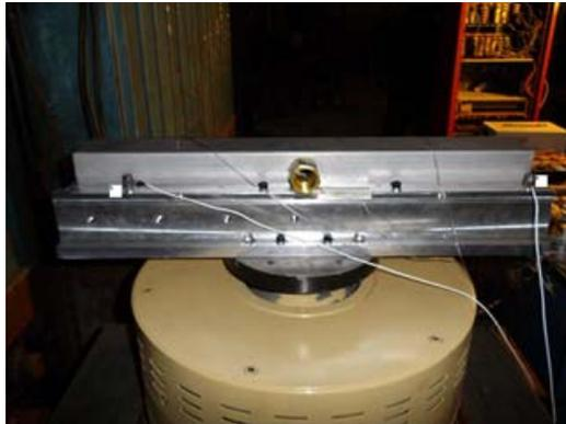
**Figure 9: Actuation system installed on cylinder for vibrational testing**
