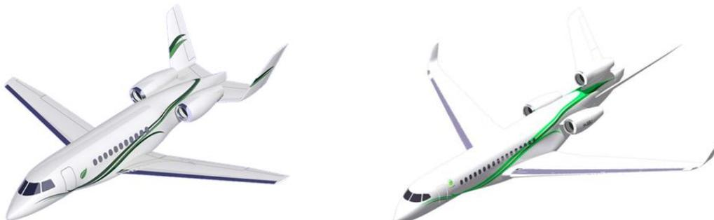
**Figure 10: Low Speed U-tail (left) and high speed V-tail**
