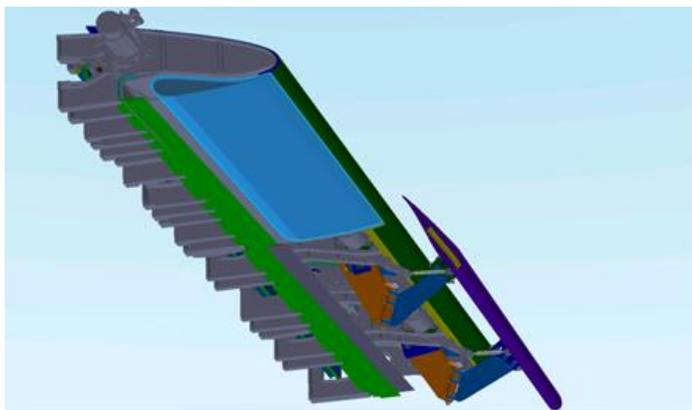
**Figure 4: Outboard Krueger flaps in retracted and deployed positions**
