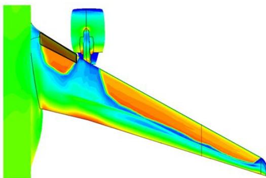
**Figure 6: HLFC suction system to laminarize the flow between engine & fuselage**
