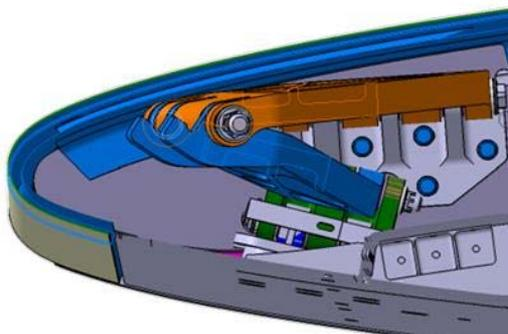
**Figure 3: Integration of the Krueger mechanism**
