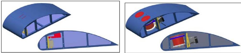
**Figure 7: Two final designs for lab model fabrication of vortex generators embedded in a typical flap**
