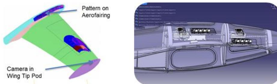
**Figure 14: (a) Reflectometry integrated in laminar wing, (b) cameras in wing tip pod**
